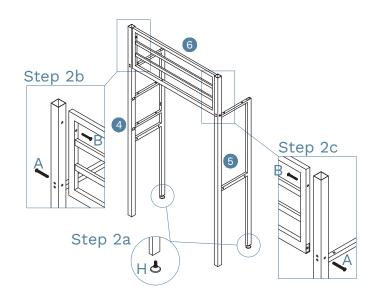
Step 2a: Attach 1 x adjustable feet (H) into panel as shown.
