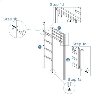
**Step 1a:** Attach 1 x adjustable feet (H) into panel as shown.
