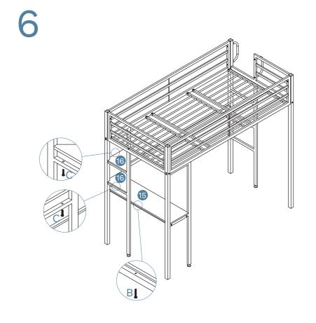
Attach 1 x bolt (B) to panel (15) and 2 x bolts (C) to panels (16) as shown. Once assembled lift furniture into place, do not drag. Ensure unit is balanced and steady before use. You're done, enjoy!
